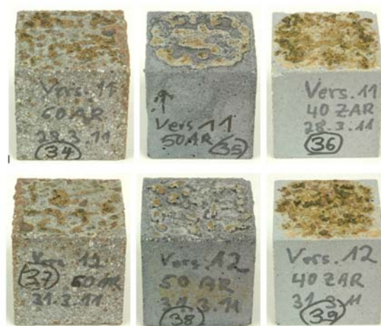
Figure 6–14 Tested material cubes 60 AR, 50 AR, 40 Z AR with BPD (standard conditions [top], oxyfuel conditions [bottom])
