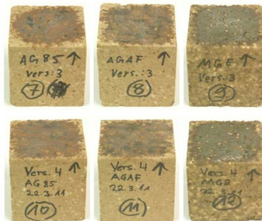
Figure 6–10 Tested material cubes of AG 85, AG AF, MG E with SCR (standard conditions [top], oxyfuel conditions [bottom])
