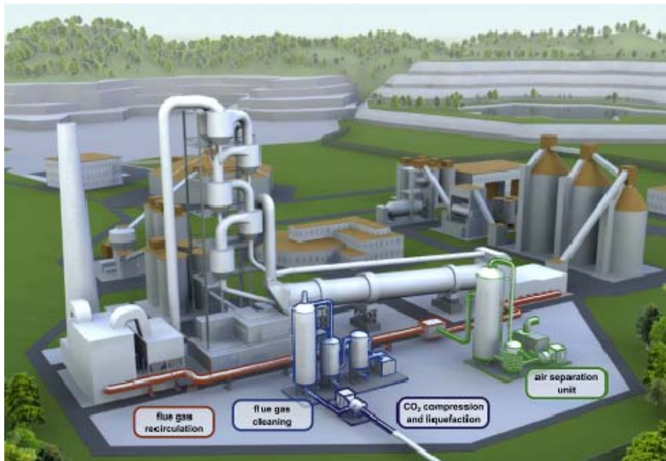
Figure 6–1 Principle of an oxyfuel cement plant
