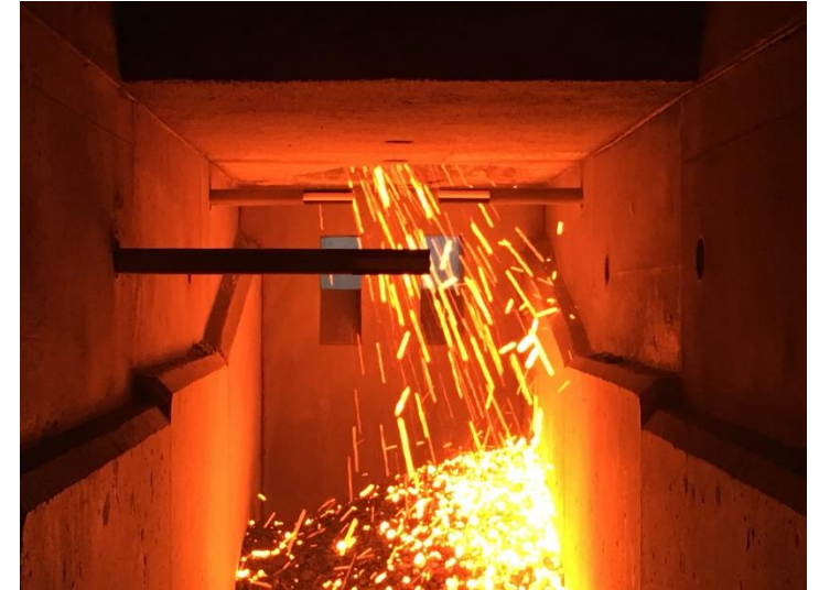
Oxyfuel clinker cooler prototype testing
