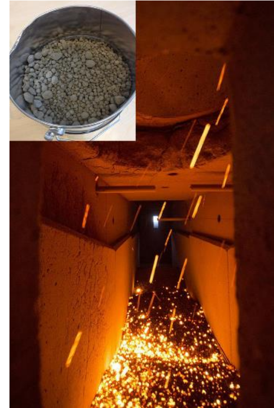
Hot commissioning of the oxyfuel clinker cooler and first oxyfuel clinker samples
