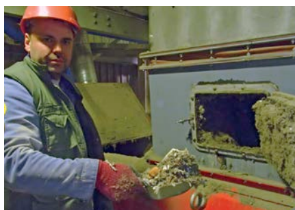
Figure 3: Sampling of alternative fuels during the verification plant tests.
