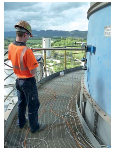
Figure 2: The verification test at two cement plants included direct CO 2 emission measurements at the stack.
