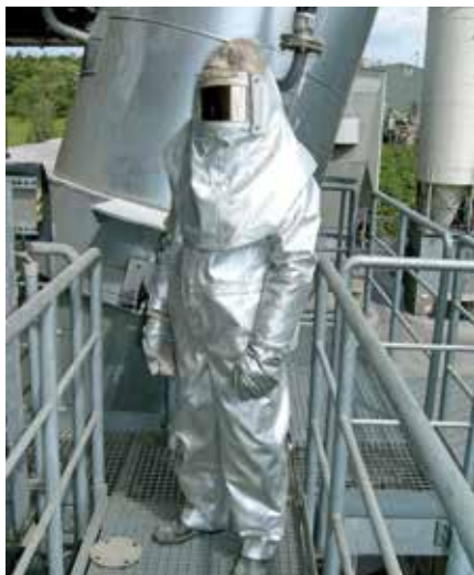
Figure 3: Suit for use when there is a high risk of meal escape.
