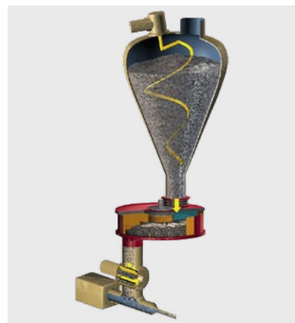
Fig. 3: Example of a feeding system for solid alternative fuels (Source: FLSmidth Pfister)
