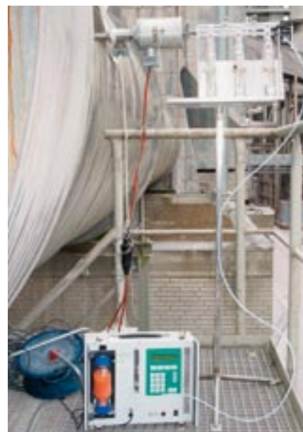
Fig. 3: Sampling of volatile chlorine, sulphur or heavy metal compounds
