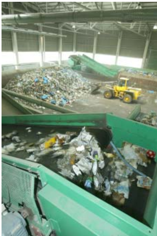
Fig. 2: View on a typical intake material for a pretreatment plant gaining alternative fuels from municipal wastes
