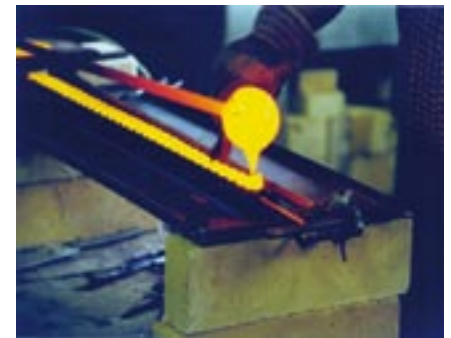
Fig. 3: Pilot trial for manufacturing compact glass pellets
